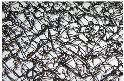
FIGURE 2. Sample of a polymer mat that is produced by making use of coiling of polymer filaments that fall onto a moving surface.
